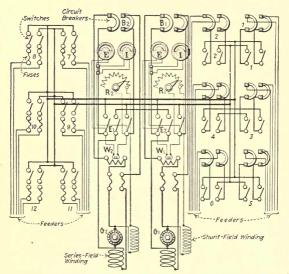
Fig. 216.—Wiring diagram for the five-panel direct-current switchboard.
